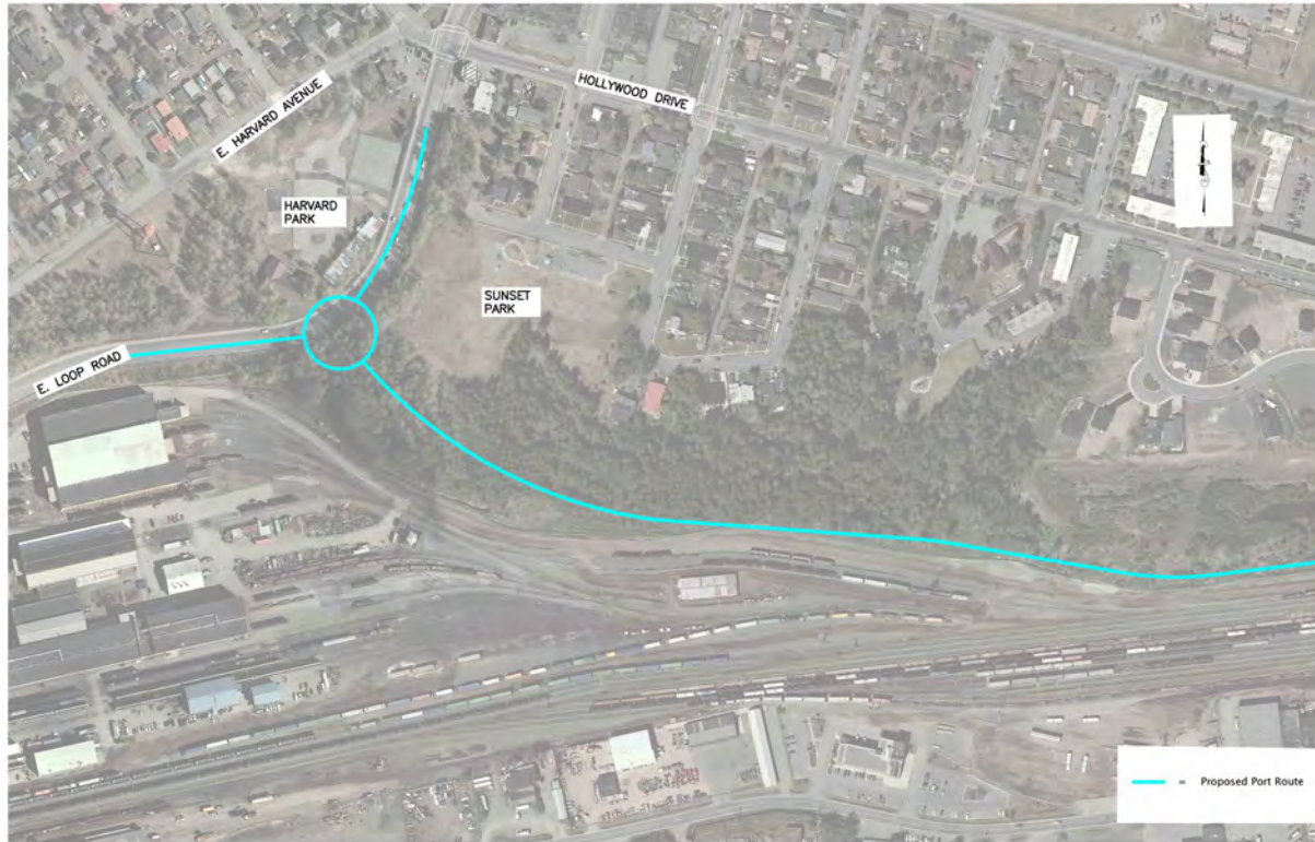
Figure 18. Potential Roundabout at East Loop Road
